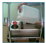
Fill the tank with water using the funnel: max. 4 ltr.
